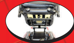
Flip-up seat for battery access
